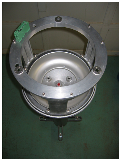
(Photo 2-2 Gauge frame on Pedestal)
