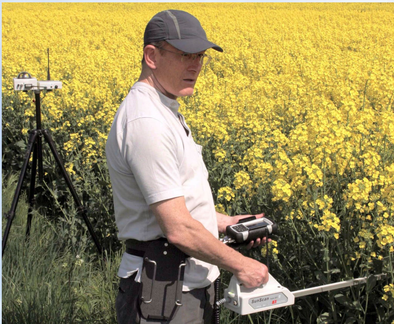
SunScan Probe (radio version) and PDA, with radio-linked BF5 Sunshine Sensor mounted on tripod
