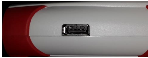
Figure 3-3 USB Port (on Left Side) of StarBright Meter
