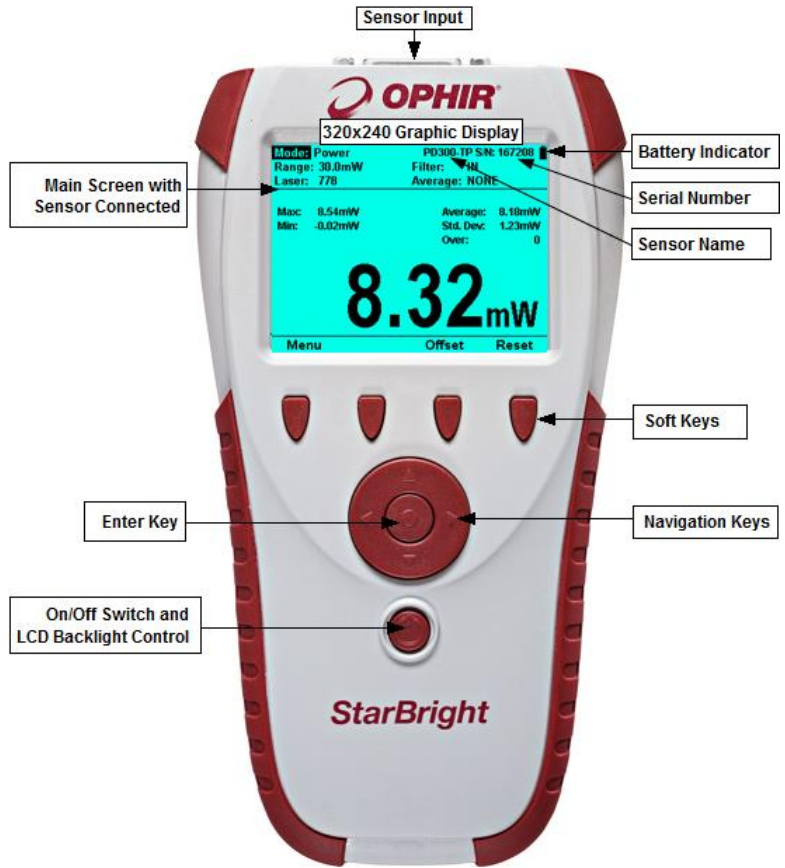
Figure 3-1 StarBright Meter/Display Unit – Front View
