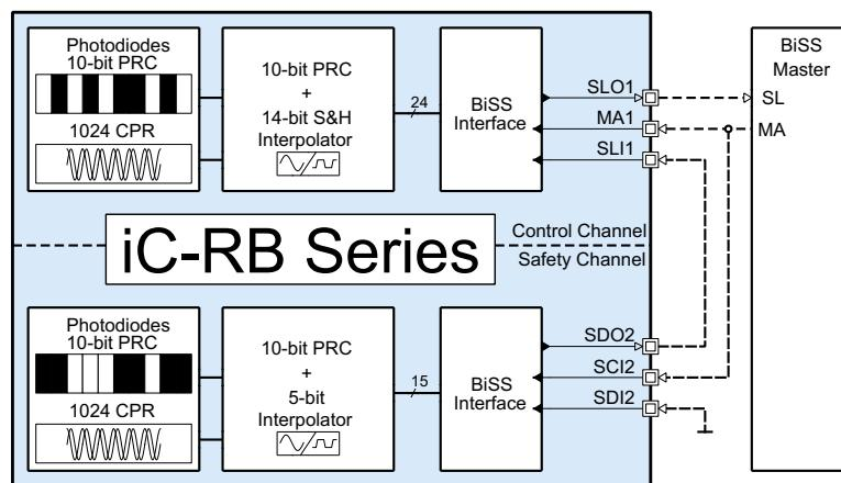
24-bit single-turn encoder with safety channel
