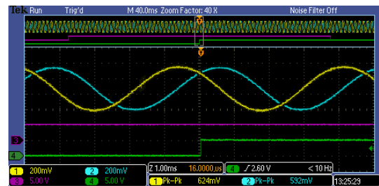
Figure 2: Regular Gray code output at MTA (CH3, magenta) and MTB (CH4, green) during normal operation; shown with PS_M (CH1, yellow) and PC_M (CH2, blue).
