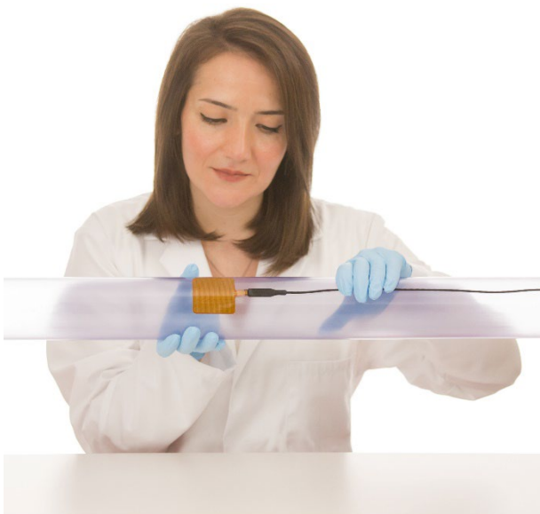
Figure 2 FHF05SC-50X50 being installed to measure heat flux on a curved surface.
