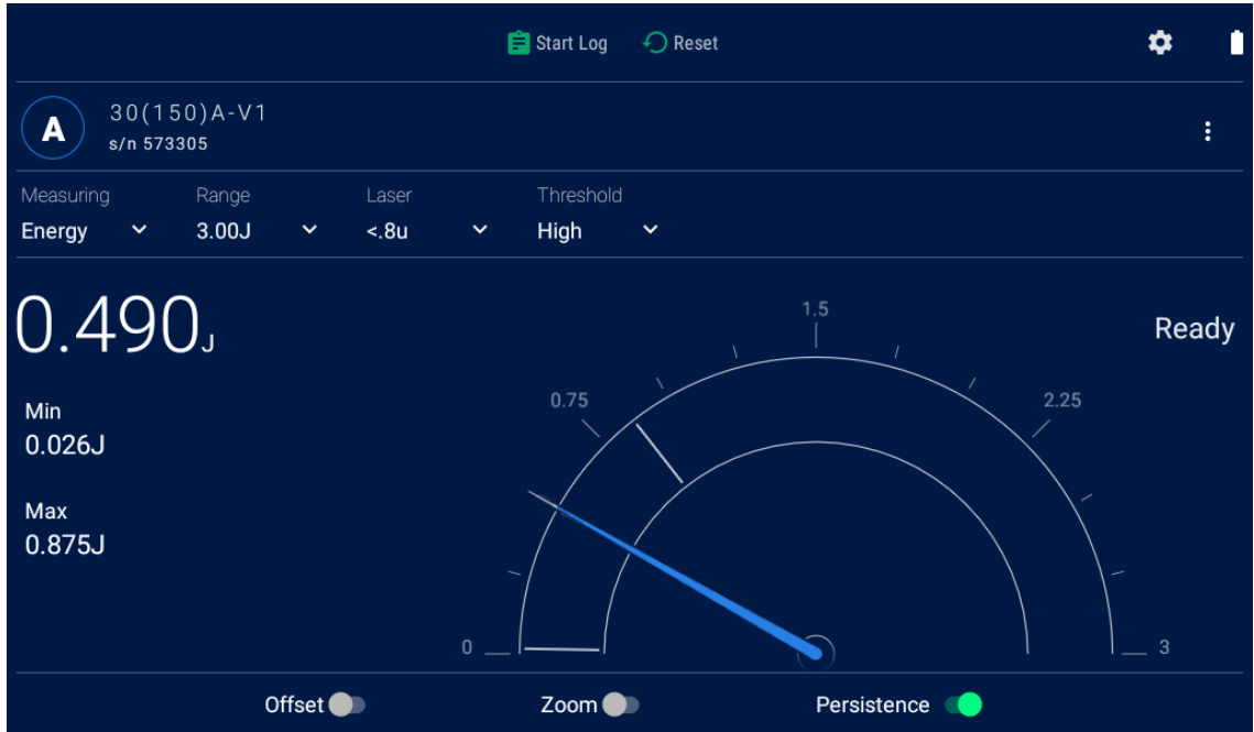
Figure 5-3 below shows a sample analog Needle display showing laser energy measurement data with options for Zoom , Offset , and Persistence . (Click the above links for more details.)
