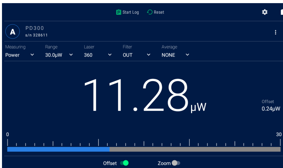
Figure 3-22 Photodiode Bargraph showing stored offset
