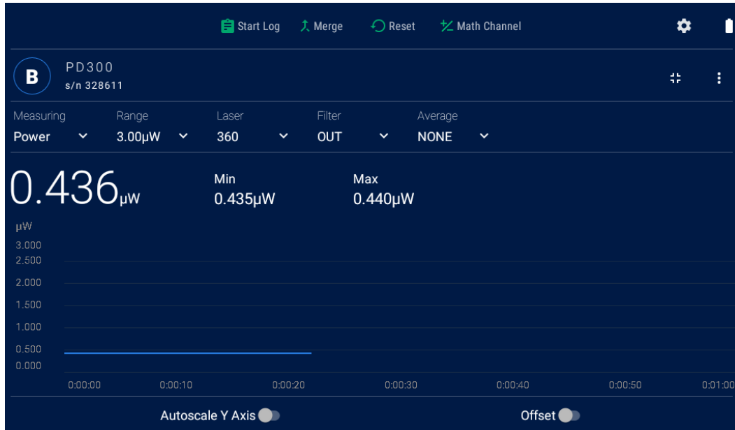
Figure 11-5 Dual Channel Operation with focus on Channel B
