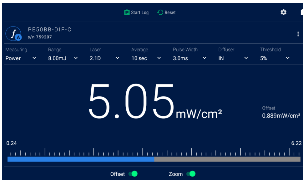
Figure 8-2 Pyroelectric Power Bargraph
