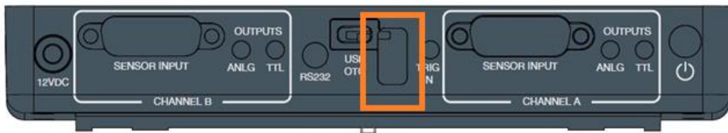
Figure 3-20 Upper panel of Centauri Meter with USB input highlighted
