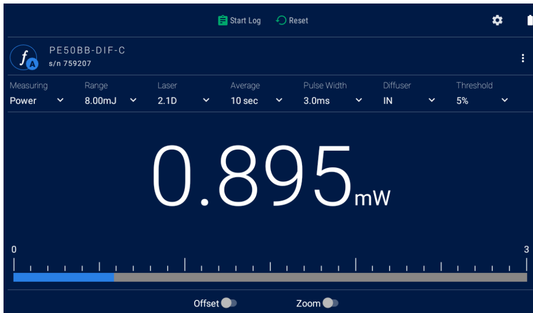
Figure 9-1 Pyroelectric Power Bargraph
