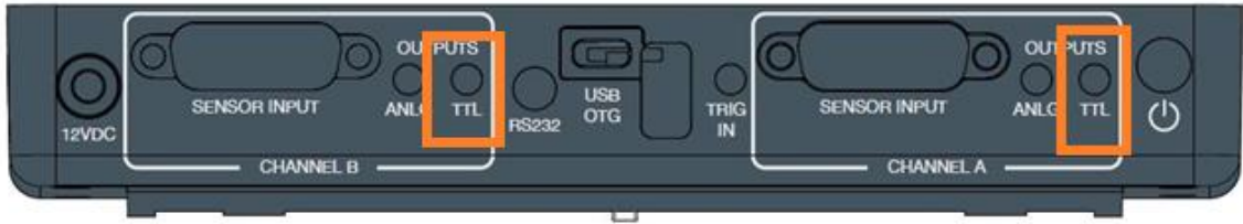
Figure 3-12 Centauri Upper View with TTL Output highlighted
