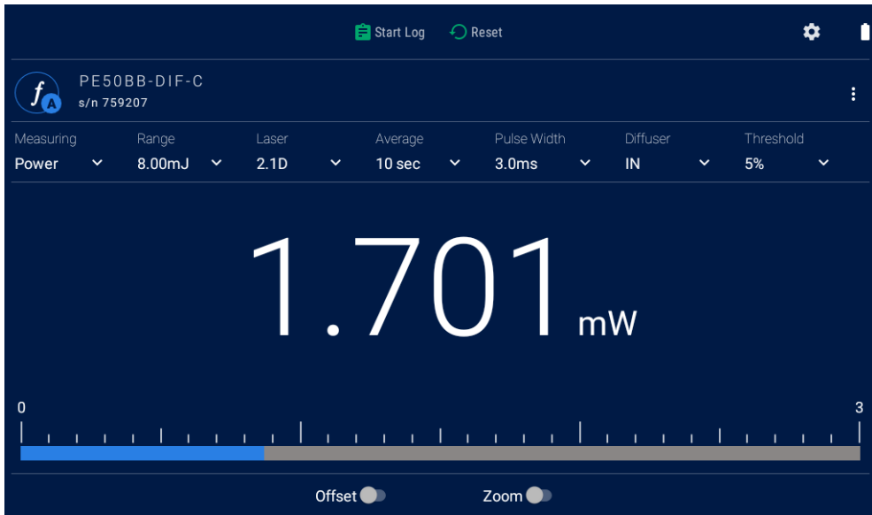
Figure 9-2 Pyroelectric Power Bargraph
