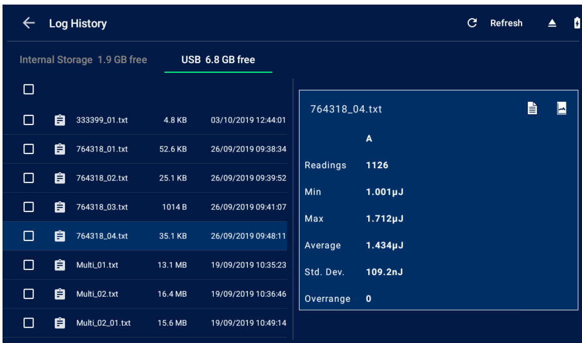
Figure 12-1 List of Log Files saved on an external storage device
